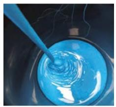
Dual-cure photoemulsions are based on newer technology and offer the largest variety in features and applications. Their main benefit is to offer high resolution and the widest exposure latitude of the three emulsion systems. Whether you need an emulsion with high chemical resistance or one specifically for glass industry, our range provides the right emulsion for your requirements.
